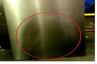
Figure-1: Typical Black Patch Defect of Cold Rolled Sheet
