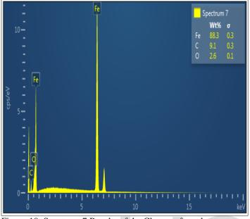
Figure-10: Spectrum-7 Results of the Clean surface sheet
