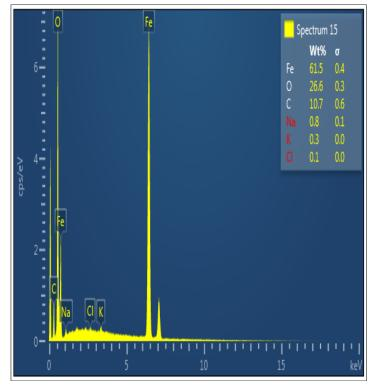
Figure 7: Spectrum-15 Results of the Black Patch surface sheet
